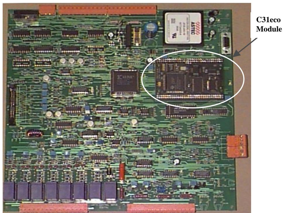
Fig.2- View of the DSP-based control PCB
