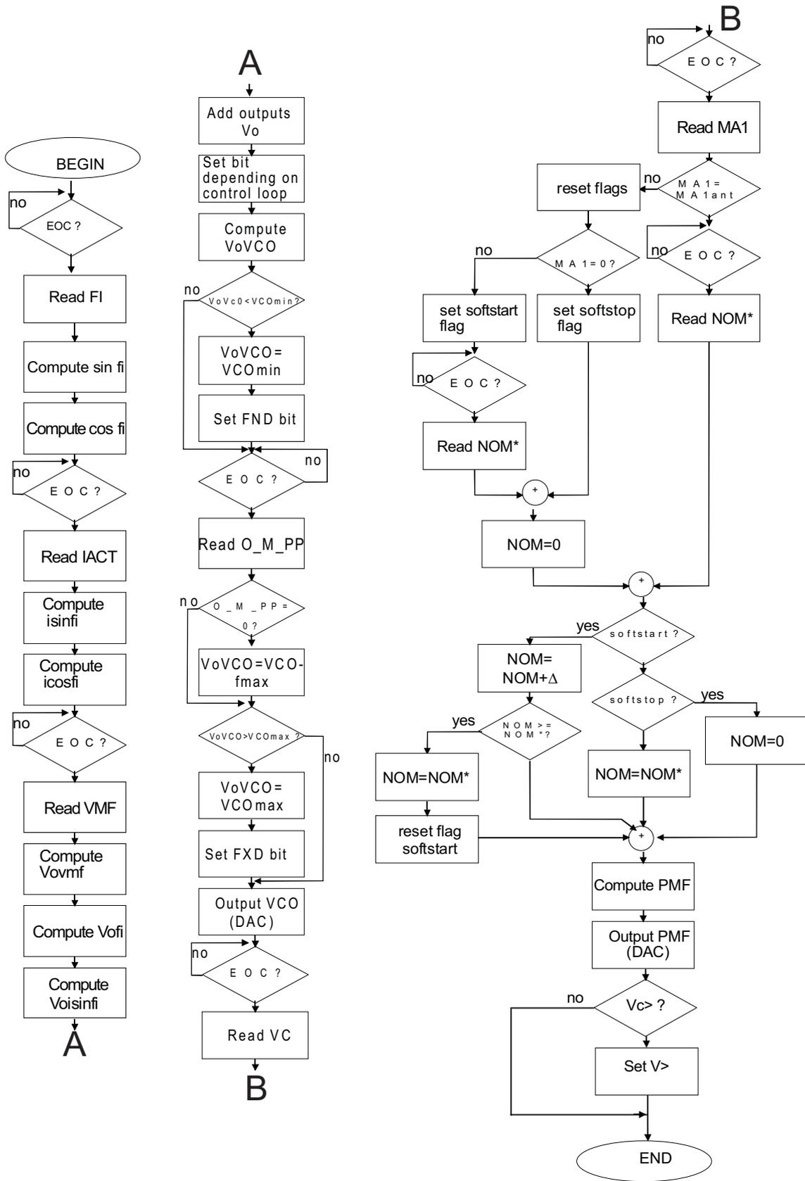
Fig.3- Flow diagram of the control algorithm
