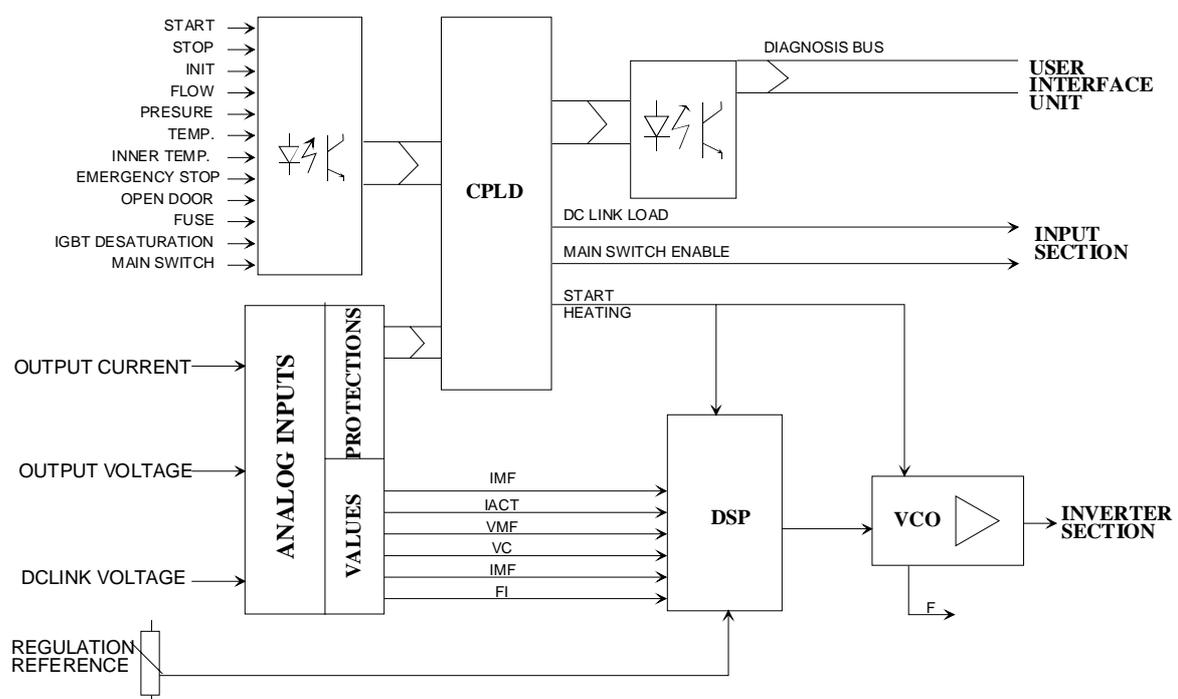
Fig.1- Block diagram for the digital control
